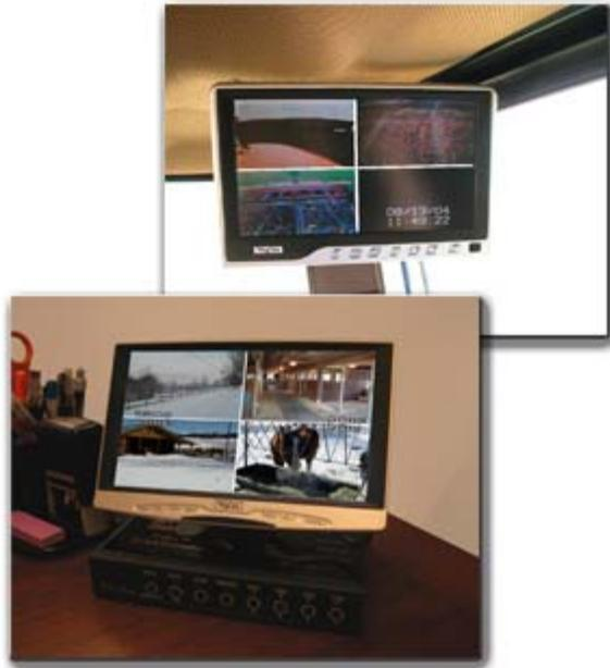
Quad will supply power to 4 cameras and output to standard TV or VCR using the RCA outputs on back and can be used without the AgCam system.
